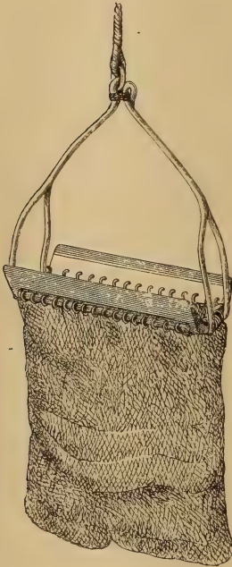
FIG. 200.—BALL DREDGE. (AFTER WYVILLE THOMSON.)
